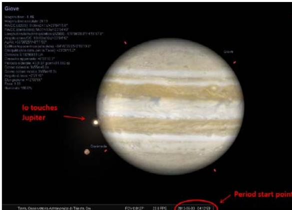
Fig. 3: Example of start point for the computation of the revolution period of Io around Jupiter.
